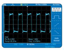
Automatically detects sine waves, square waves and video signals, with readouts of relevant measurements and additional user-selectable views of the signal.
