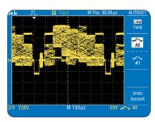
Pulse-width and field- and line-selectable video triggers make the oscilloscope ideal for a wide range of applications.
