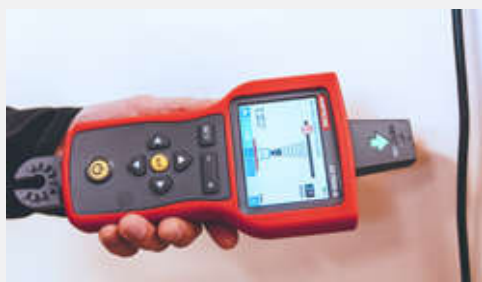
Non-contact voltage (NCV) detection.
