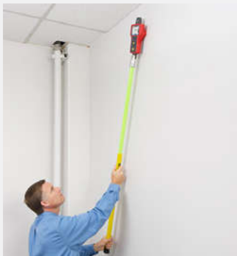
Trace wires in hard to reach places with the TIC 410A.
